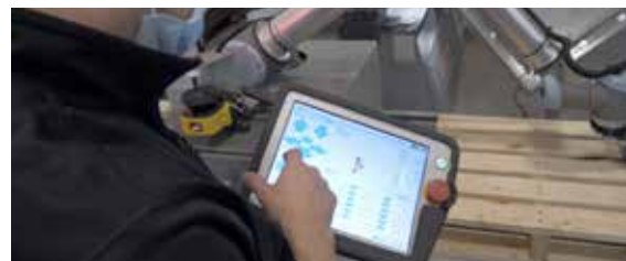
Programming the palletizing element of Siouxland Fabricating's stamping application is a cinch thanks to greatly simplified and highly graphical 'Palletizing Wizard' developed by cobot pioneer Universal Robots. Credit: Universal Robots
