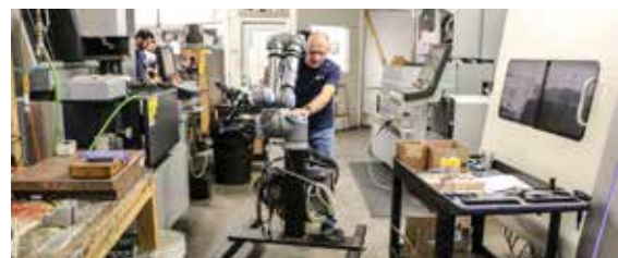
All Axis Machining developed a mobile platform so that its cobot can quickly be moved through the facility and deployed on different applications. Credit: Universal Robots
