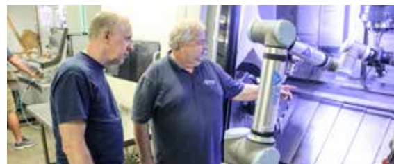
Easy communication between old equipment and a cobot from Universal Robots enabled All Axis Machining to completely automate several machine tending processes. Credit: Universal Robots
