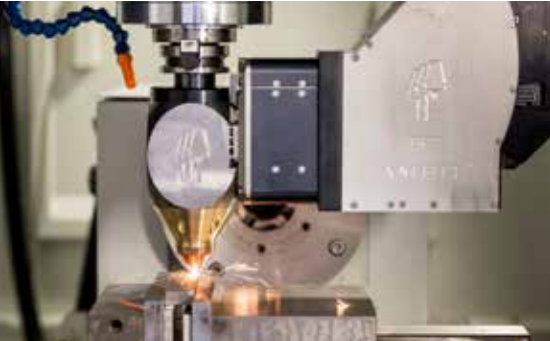
With the AMBIT FLEX, a dockable tool carousel enables interchanging tools for different deposit widths or metals.
