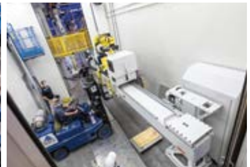
The Auto-SLC uses a laser to ablate the surface around the holes where nutplates are bonded, removing any surface impurities which may taint the bonding surface.
