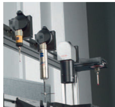
The ability to perform tactile, optical and laser measurements with the same base system can eliminate the cost of multiple machines
