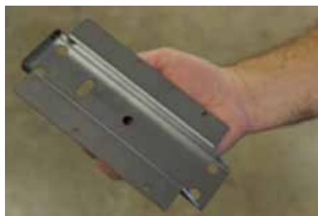
The robotic press brake also provides consistent bends, enabling the equipment to meet high tolerances repeatedly.
