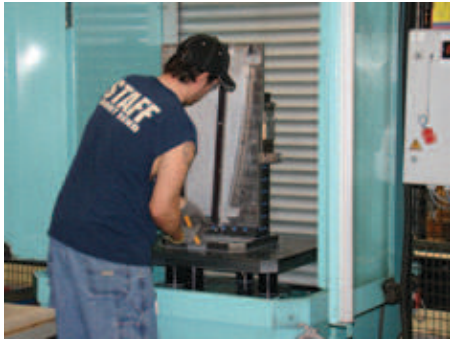
A Steelville Mfg. worker loads parts into a tombstone for machining in the Fastems cell.
