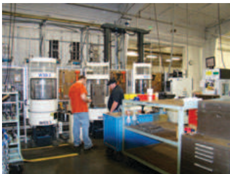
SMC's MMC automated pallet-delivery work cell has three workstations
